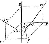
sects the axis of Y, draw a parallel to the axis of X: then will P be the projection of the point (P', P''), on the coordinate plane YX.
